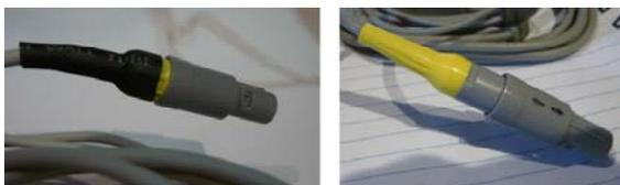
Figure 1 – Improved probe connectors
